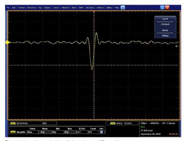
Pinpoint triggering can isolate glitches down to 100-ps wide
