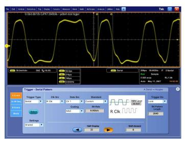
NRZ Pattern Lock Triggering of a 640-bit long SATA serial pattern at 6 Gbps
