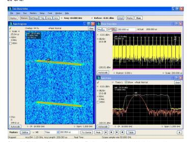
SignalVu™ Vector Signal Analysis – Easily verify wide-bandwidth designs such as wideband radar, high data rate satellite links, or frequency-hopping radios and characterize wideband spectral events. SignalVu combines the functionality of a vector signal analyzer, a spectrum analyzer, and the powerful triggering capabilities of the DPO/DSA70000B – all in a single package.
