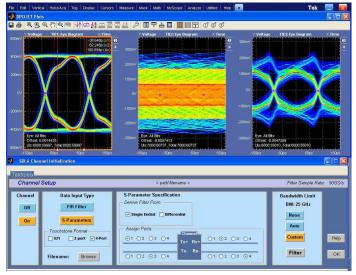
SDLA - Serial Data Link Analysis (options SLE and SLA) - Gain insight into serial data links with the capability to emulate the serial data channel from its S-parameters, de-embed the fixture or other network, and add or remove transmitter equalization (de-emphasis/pre-emphasis). Option SLA adds processing of waveforms with FFE and DFE equalizations and automatic equalizer training. DPOJET provides advanced measurement and jitter analysis of the resulting waveforms.
