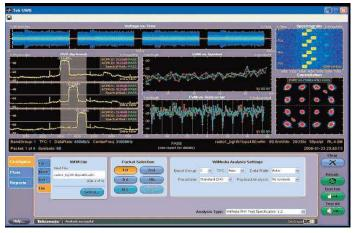
Ultra-Wideband Spectral Analysis Software (Opt. UWB) – Analyze hundreds of packet, TFC, and data-rate combinations without adjusting the UI. In addition, the automatic WiMedia modulation analysis configuration will analyze how complex wideband signals change frequency and amplitude with time using real-time spectrograms spanning 20 GHz.
