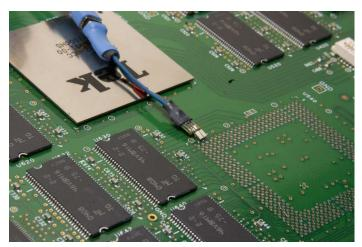
Low-cost solder tip features quick connection so moving probe to various solder points is
