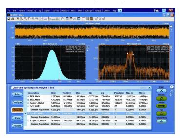
DPOJET Jitter And Eye Diagram Analysis (Opt. DJA) – Simplify identifying signal integrity concerns, jitter, and their related sources with DPOJET software. DPOJET provides the highest sensitivity and accuracy available for real-time oscilloscopes.
