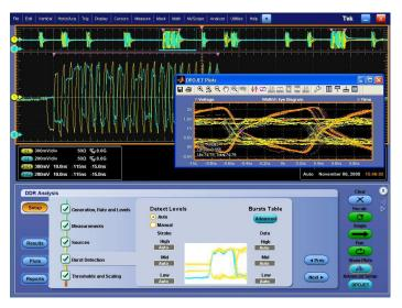
DDR Memory Bus Analysis (Opt. DDRA) - Automatically identify DDR1, LP-DDR1, DDR2, DDR3, and GDDR3 Reads and Writes and clearly see and analyze how analog anomalies are affecting your DDR/Memory. DDRA with DPOJET, combined with the DPO/DSA70000B DPX® technology, is the fastest way to solve complex memory signaling issues.
