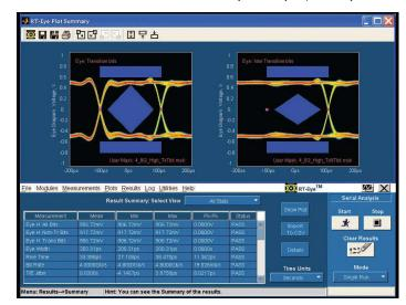
**FB-DIMM Compliance Test Solution (Opt. FBD)** – Test the Receiver, Transmitter, and Reference clock test points for compliance as per FB-DIMM standards.
