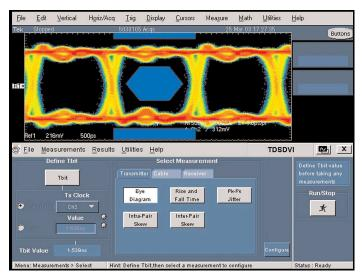
**DVI Compliance Test Solution (Opt. DVI)** – Obtain quick and dependable results with the DVI compliance test software. Automated testing based on objective pass/fail detection without human intervention will dramatically enhance your productivity.
