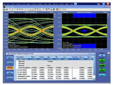
**USB 3.0 Transmitter Testing** – Verify, debug, and certify to the specifications of the USB 3.0 PHY layer using native capabilities in and additional applications for the DPO/DSA70000B series. Math function FIR filters and SDLA software, allow emulation of the Cable and Reference channels defined in the USB 3.0 spec. With DPOJET, jitter measurements needed to complete the Normative compliance test can be done.
