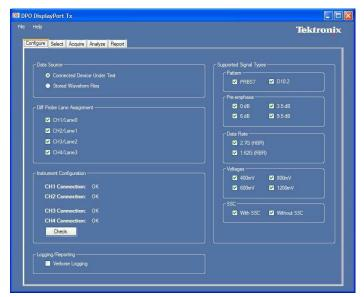
**DisplayPort Compliance Test Solution (Opt. DSPT)** – Support DisplayPort Compliance Test Standard (CTS) source test with four-line simultaneous testing using the Tektronix P7300SMA Series probes and DisplayPort software. Detailed test reports with waveform plots, pass/fail results, and margin analysis are included.
