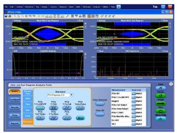
PCI Express Analysis Test Solution (Opt. PCE) - Analyze the performance of your PCI-Express Rev 1.0, 2.0, or 3.0 (draft spec) design with comprehensive test support. Option PCE enables tests that conform to PCI-SIG standards using either DPOJET or RT-Eye.
