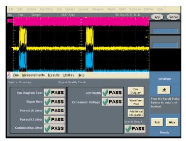
**USB 2.0 Compliance Test Solution (Opt. USB)** – Ensure your design has sufficient margins by characterizing your device with variable test limits. The USB compliance test solution provides "one touch" compliance testing by automatically setting up the oscilloscope for all compliance test configurations including probe deskew.
